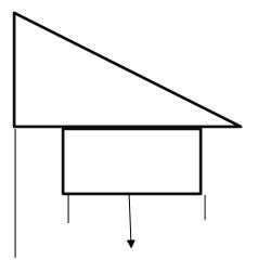
Iron ore falls steadily under gravity onto a conveyor belt at a rate of 40 tones a minute. What force is needed to maintain a speed of 1.6m/s in the conveyor belt?
