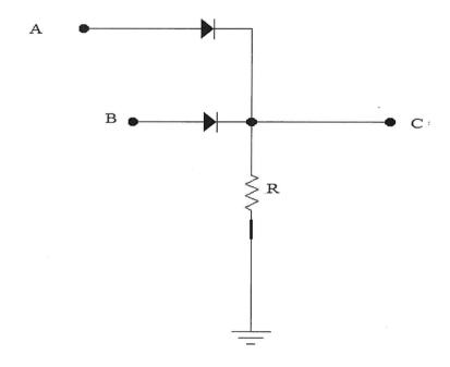
(I). Identify the gate and provide its corresponding logic symbol.
