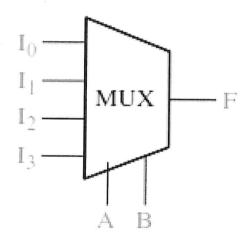
The control inputs select which one of the data inputs is transmitted to the output. The logic equation for the 4-to-1 MUX is  $\mathbf{F} = \mathbf{A'B'I0} + \mathbf{A'BI1} + \mathbf{AB'I2} + \mathbf{ABI3}$ . Use the VHDL statement to model the MUX. (7marks)
