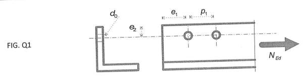
Given the single angle  $60 \times 60 \times 6mm$  steel grade S275 with a two M16 bolts in Fig.Q1 where  $p_1=45mm$ ,  $e_1=50~mm$ ,  $e_2=30~mm$ , d=16~mm, Applied force  $N_{Ed}=75~kN$ . Check for the adequacy for the following
