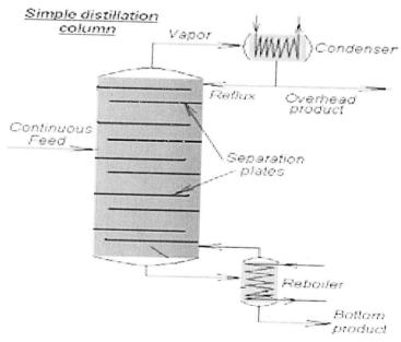
If we feed the column with a liquid of components A and B that have boiling points  $T_A$  of 40 °CF and  $T_B$  80°C for components A and B respectively;
