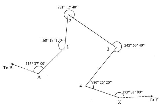
Given the lengths of the traverse legs as shown in the table below, calculate the coordinates of stations 1,2,3,4, adjusting any misclosure by the bowditch method.
