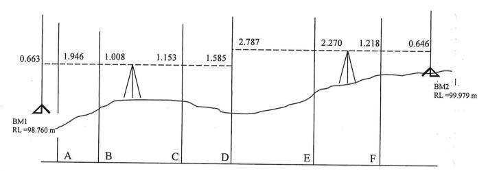
Determine the reduced levels at the various staff stations by the Rise and Fall Method, applying the necessary arithmetical checks. (10 marks)
