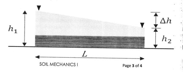
e) For a variable – head test, the following results were obtained. Length of specimen = 380 mm, area of specimen = 6.5 cm<sup>2</sup>; k=0.175 cm/min. determine the area of the standpipe for the head to drop from 650cm to 300 cm in 8 minutes. [4 Marks]
