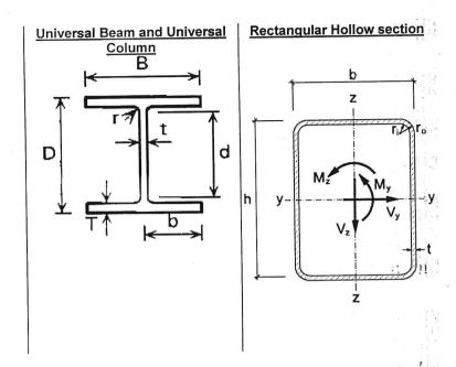
Section properties Universal Equal Universal Column Angle Beam 60x60x5 305x305x97 406x140x46 4.57 kg/m 46.0 96.9 Mass per metre 307.9 60 403.2 h mm Depth of section 60 142.2 305.3 b mm Width of section 1.64 С mm
