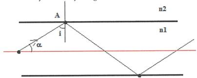
i) Find the refractive index  $n_2$  of the cladding so that the critical angle at the interface core cladding is 80 °.
