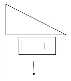
Iron ore falls steadily under gravity onto a conveyor belt at a rate of 40 tones a minute. What force is needed to maintain a speed of 1.6m/s in the conveyor belt?
