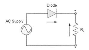
Calculate the equivalent DC voltage developed across the load, the load current and power dissipated by the load. Assume ideal diode characteristics. Find the following:
