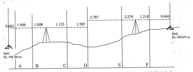
Determine the reduced levels at the various staff stations by the Rise and Fall Method, applying the necessary arithmetical checks.
