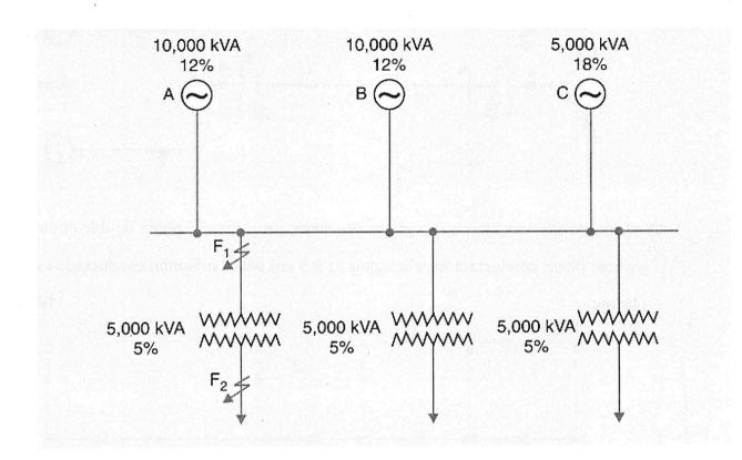
Determine the maximum fault MVA which the circuit breakers on;
