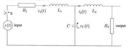
Taking the resister  $R_1$  current as the state  $x_1(t)$ , the inductor  $L_2$  current as the state  $x_2(t)$ , the capacitor voltage as state  $x_2(t)$ , e(t) = u(t) and output voltage is y(t). Given that  $R_1 = 8\Omega$ ,  $L_1 = 0.25H$ ,  $R_2 = 4\Omega$ ,  $L_2 = 0.5H$ , C = 1F, assuming that the switch S is closed at time t = 0.
