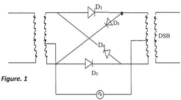
The circuit of Figure 1 is a Ring Modulator. Describe its Principle of Operation.
